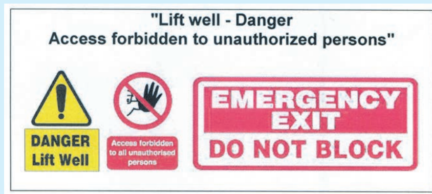
FIG. 6 TYPICAL NOTICE ON ACCESS DOORS AND EMERGENCY DOORS
