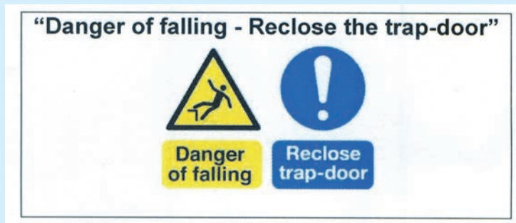
FIG. 5 TYPICAL NOTICE ON TRAP DOORS
