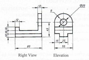
6B. Draw the axonometric projection of an object whose orthographic projections are as shown in Fig below. All dimensions are in mm.
