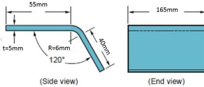
A Sheet metal is bent as shown in the above figure. Find the Starting blank size of the sheet metal. Use  $K_{ba}\,{=}\,0.33$
