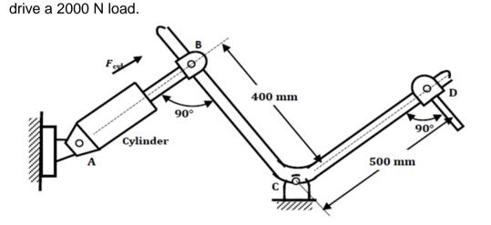
For the system given in the figure below, determine the force required to
