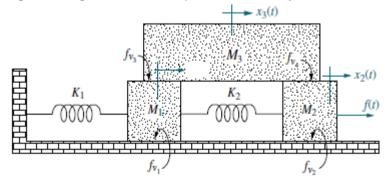
2A. Find the equivalent transfer function, T(s)= C(s)/R(s), for the system shown in (04) Figure
