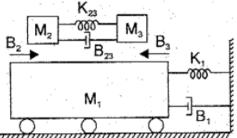
**1C.** Write down the governing differential equation of the system shown below **(02)**
