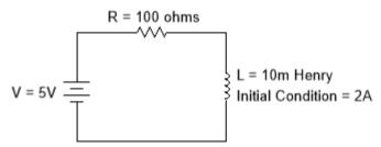
If the initial current in the inductor is 2A, what is the current through the inductor at time t = 0.2 milliseconds?
