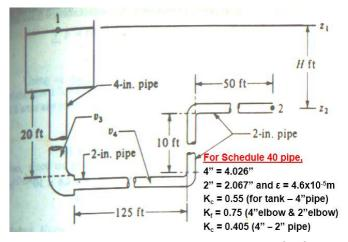
4B. Water at 20°C is being pumped from a tank at the rate of  $5 \times 10^{-3} \text{ m}^3/\text{s}$ . All of the piping is 4" schedule 40 pipe. The pump has an efficiency of 65%. Calculate the kW power needed for the pump. Given that for 4" Schedule 40 pipe, D=0.1023m, Kc=0.55, Density = 998.2 kg/m<sup>3</sup>, K<sub>f</sub>=0.75, Viscosity=1.005 cP, Kex=1.0, f=0.0051. Mention the assumptions if any. (10)
