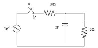
In the network shown, the switch is moved from a to b at t=0, Determine  $v_c(t)$
