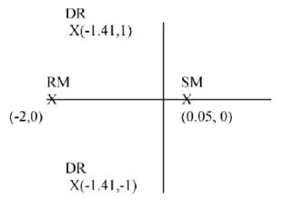
Determine the time constant for the dutch roll (DR), spiral mode (SM) and roll mode (RM). Also determine the natural frequency and damping ratio of the dutch roll mode.
