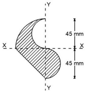
Determine moment of inertia of the shaded area shown in (2) the figure with respect to a given reference axis AB. A)
