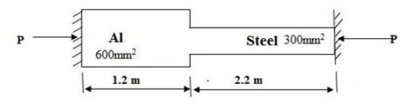
6C) Determine the total compression of the bar shown in the (6) figure. Take  $E_{st} = 210$  GPa,  $E_{br} = 105$  GPa and  $E_{cu} = 100$ GPa
