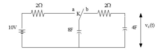
Determine the source current when the switch K is closed (10) at t=0.Assume zero initial conditions
