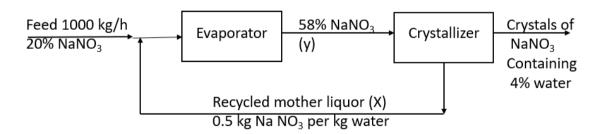
Calculate i) the yield of crystals ii) the mass flow rate of the recycled mother liquor iii) the composition of the mixed feed entering the evaporator and iv) the total feed rate to the evaporator. (All percentages are by weight).
