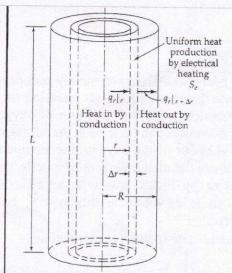
Heat conduction with an electrical heat source is shown in the figure. Using shell balance technique, Develop a mathematical equation which gives the temperature profile from the center of the wire to the surface of the wire.
