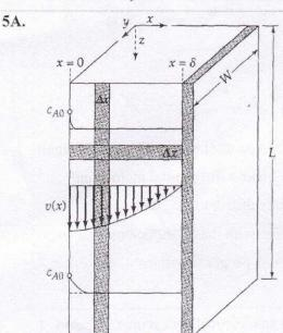
Absorption of A (gas) into a falling film of liquid B is shown in the figure. Using shell balance technique, Develop a mathematical equation to show the concentration gradient in x direction
