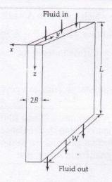
A newtanian fluid is in laminar flow in a narrow slit formed by two parallel walls a distance 2B apart. It is understood that B<<W, so that edge effect are unimportant. Make a differential momentum balance, and obtain the expression for momentum flux and velocity distribution
