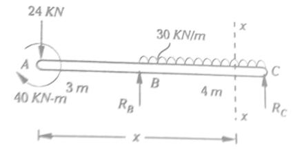
3) For the beam configuration shown in figure determine the deflection and slope at the free end using direct integration method.
