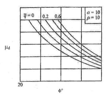
Design charts for nailed walls and slopes with L/H = 0.6 by Gassler, 1996
