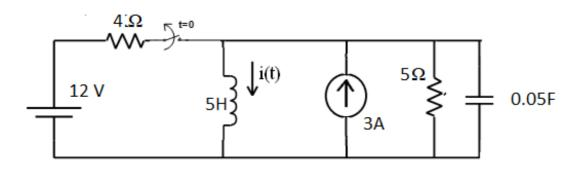
B) The switch in figure below was open for long time but closed at t = 0. Determine (a) i(0+), v(0+) (3) (b) di(0+)/dt. dv(0+)/dt (c)  $i(\infty), v(\infty)$ .
