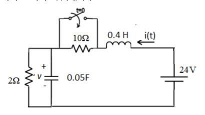
C) Assuming that the switch shown in figure below has been in position A for a long time is moved to (2) position B at t = 0. Find Vo(t) for  $t \ge 0$ .
