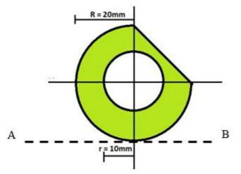
C) Find the Moment of Inertia and radius of gyration of the shaded portion about <sup>(4)</sup> AB.
