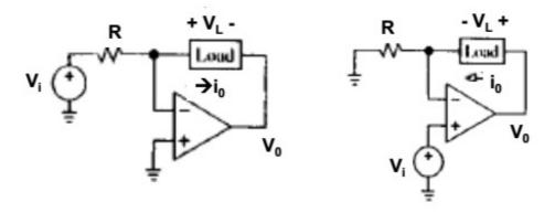
4) Obtain component values of the following circuit for a unity-gain frequency of 100 Hz: (2)
