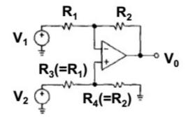
3) Compare the V to I circuits in Figures. Calculate i<sub>0</sub> in both cases and find out the voltage compliance and maximum permissible value of load resistance.
