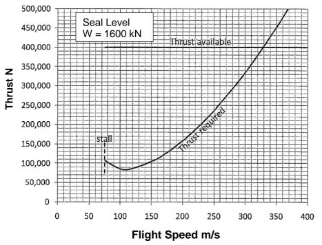
Using the above data calculate C<sub>Lmax</sub>, (L/D)<sub>max</sub>, C<sub>D0</sub> and k for the aircraft. **1B** Obtain the percentage throttle setting required for a steady level flight at sea level [02] flight at M = 0.8. (at sea level a = 340.29 m/s).
