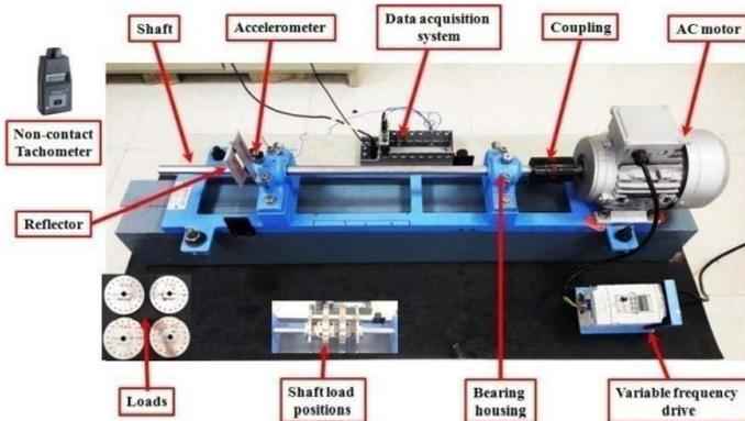
Fig. Q1b: System components for condition monitoring
