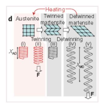
Methods of soft actuation for the figure can be described as
