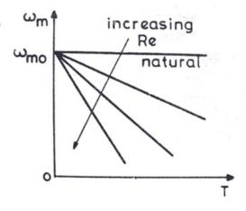
These are speed torque characteristics where the speed of the motor is being controlled by adding a resistance to the armature and varying it. This is the most reliable method amongst voltage, field flux control and armature resistance control.
