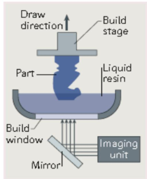
Identify the Additive manufacturing technique for the fabrication of physical objects through the successive addition of material layers as shown in the figure
