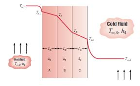
Draw the thermal circuit and write the expression for heat transfer rate in a one-dimensional flow. (2)
