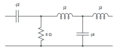
2) For the coupled circuit shown calculate the values of current and Vo
