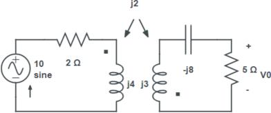
In the circuit shown the reactance and resistance associated with the load are varied. Determine ZL for it to receive the maximum power and B) (3) obtain the maximum power.
