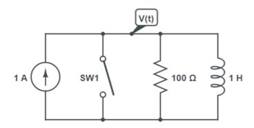
B) For the circuit shown the switch is closed at t=0 with initial zero current in inductor, calculate I, di/dt and d<sup>2</sup> i/dt<sup>2</sup> at t=0+.
