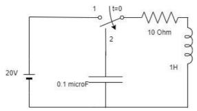
In the network shown, the switch S is opened at t=0. Solve for the voltage v(t) for  $t \ge 0$ , using the classical time domain approach. (5) Assume all initial conditions are zero. [CO2, PO 1,2, BL3]
