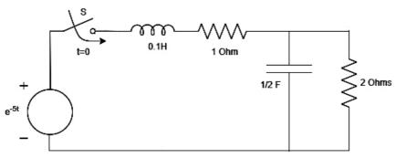
Determine voltage ratio  $V_2(s)/V_1(s)$ , Current ratio  $\frac{1}{2}(s)/I_1(s)$ , and input impedance  $V_1(s)/I_1(s)$  for the following circuit using transform (3) method. Assume all initial conditions are zero. [CO3, PO1,2, BL3]
