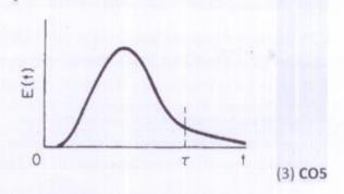
Q5B. Tracer hytane was injected as a pulse into the reactor with a flow rate of 10 dm<sup>3</sup>/min and following effluent concentration was measured as the function of time.
