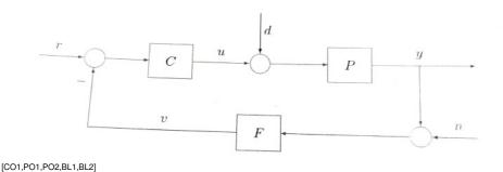
Fig.1A Control system block diagram
