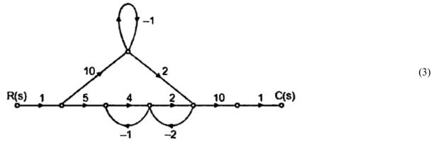
C) Reduce the Block Diagram to a Signal Flow Graph and obtain the Transfer Function C(S)/R(S)
