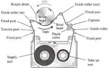
**4B.** Consider the audio tape speed control system shown in figure. Design a PD controller that will yield a peak time of 1.047 seconds and a damping ratio 0.8 for a step input.
