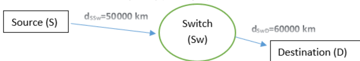
Fig Q.1B: Packets transmission through virtual circuit switching mode.
