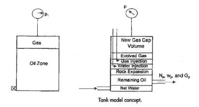
Based on the geological evidence it is known that the areal extent of an oil reservoir is 740 acres, the thickness of the pay zone is 40 ft, the porosity is equal to 30%, and  $S_w$  (water saturation) is 25%, and there is no  $S_g$  (free gas saturation). Consider  $B_{oi}$  as 1.306 bbl/STB.
