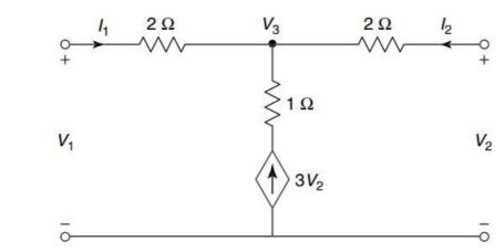
B) Develop the T parameters for a two port network.
