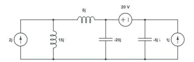
B) Analyse the coupled circuit to find current  $I_1$ ,  $I_2$  and  $V_0$
