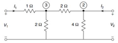
5B) Find transmission parameters for the two-port network shown in Figure. (4)
