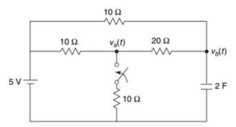
For the network shown in the Figure the switch is opened at t = 0. Find V(t) for t > 0.
