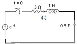
3B) Use mesh analysis to find  $v_o(t) for \ t > 0$ , in the network in shown in figure using Laplace (4)
