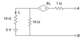
1C) For the circuit shown in the Figure find Ix using Superposition Theorem. (2)
