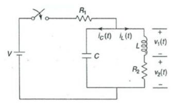
2B) In the network shown in the Figure a steady state is reached with switch open. At t = 0, switch is closed. (4)
