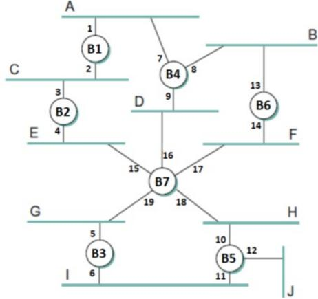
We denote a configuration message from node X in which it claims to be distance d from root node Y as (Y, d, X). For example, the first configuration message sent by bridge B7 is (B7, 0, B7). After the spanning tree algorithm converges, what are the configuration messages sent by bridge B2, B3 and B7, 4respectively?
