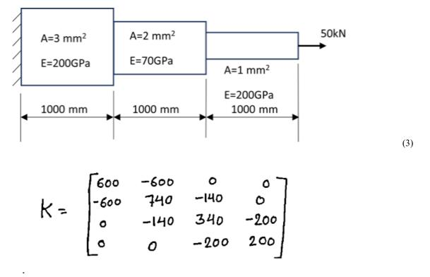
(While calculating the global stiffness matrix above, the dimensions were expressed in mm, and the unit used for force is N.)
