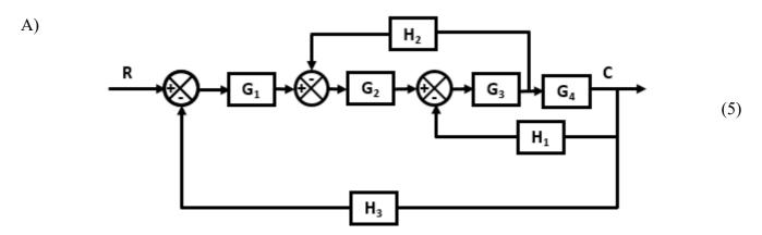
B) Draw the signal flow graph for the block diagram shown below and determine the transfer function using Mason's Gain method.
