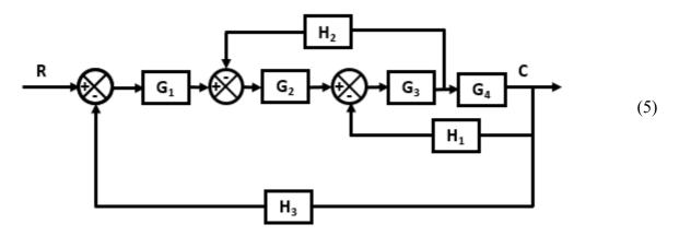
Perform the time response analysis of control system shown below for the unit impulse input signal. The value of damping ratio is i) in between 0 to 1 and ii) greater than 1. Also plot the nature of output signal.
