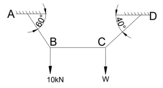
2B) Determine the support reactions for the beam shown in figure
