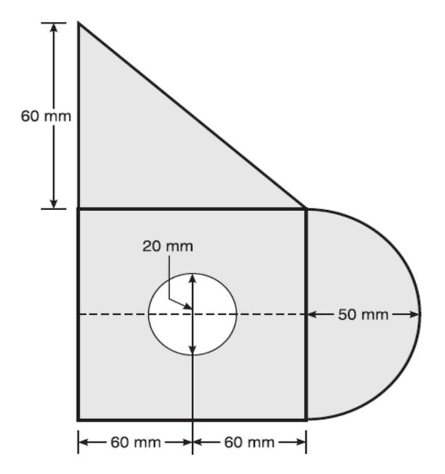
Find the moment of inertia of Figure about the centroidal vertical axis (all dimensions in (5) mm).
