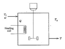
(a) Develop a mathematical model (differential and algebraic equations) that describe the exit temperature if heat losses to the ambient occur and if the ambient temperature (T<sub>a</sub>) and the incoming stream's temperature  $(T_i)$  both can vary.
