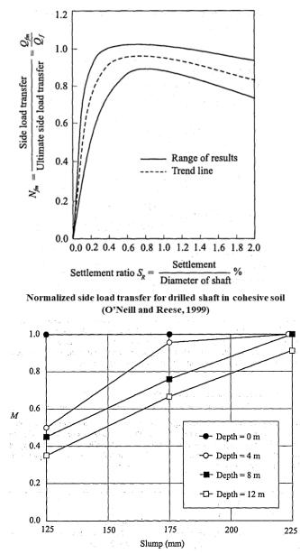
Factor M vs. Concrete slump (O'Neill et. al , 1996)
