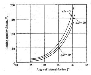
Berezantsev's bearing capacity factor,  $N_{\rm q}$  (after Tomlinson, 1986)
