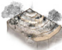
Smallest Scale: Contour Trenches, Bunds and Retention walls preventing soil erosion
